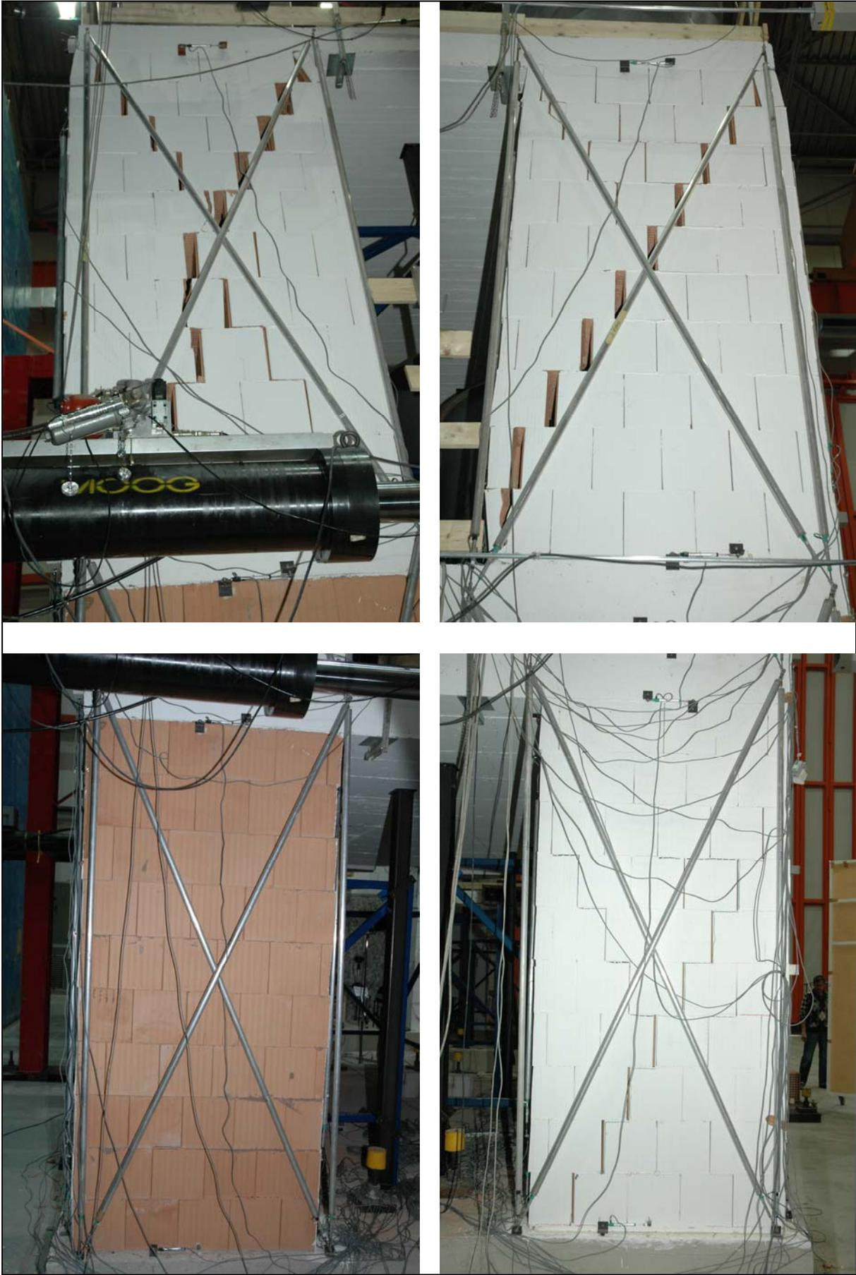
Figure 16: Damages in the slender walls after the final test (0.22g)
