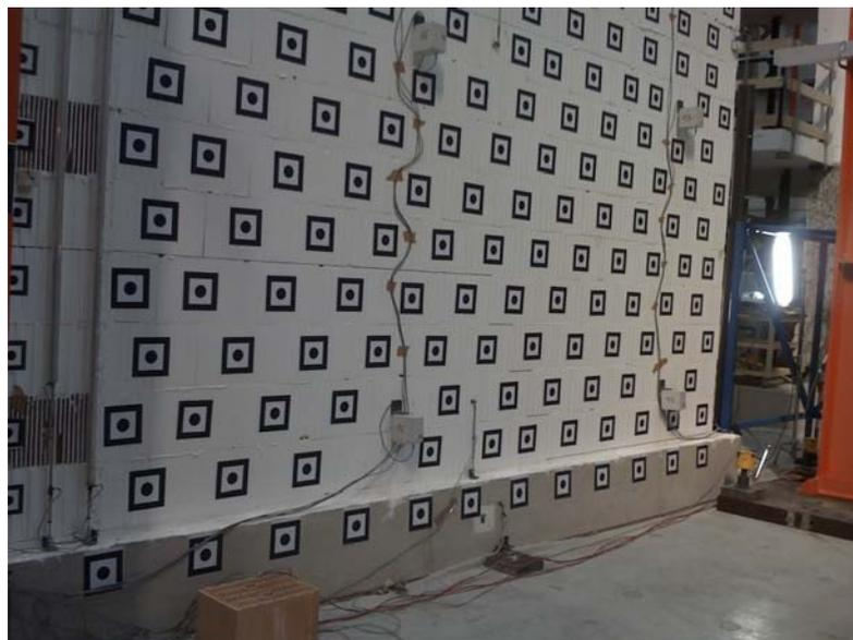
Figure 13: Flexural cracks on the east transversal wall during the 0.12g test
