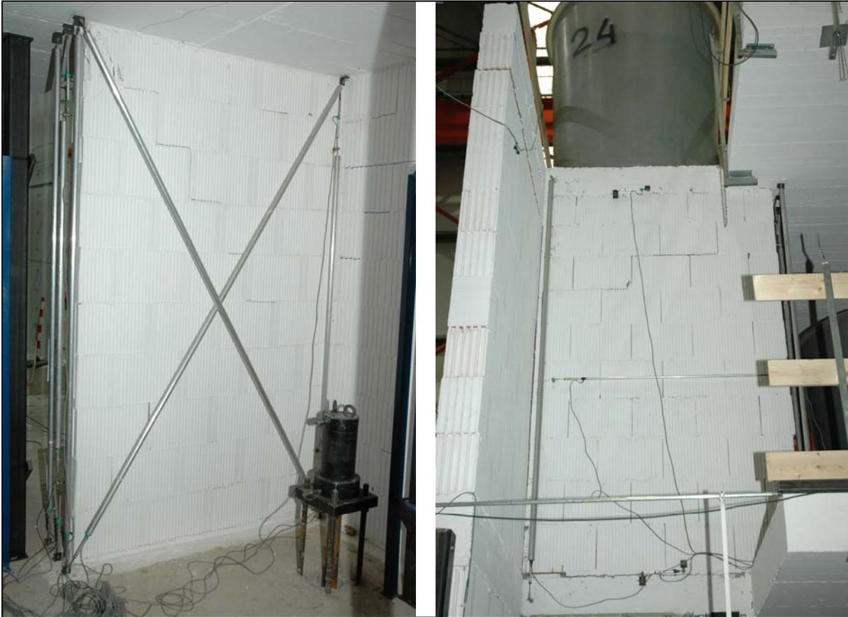
Figure 17: Damages in the main shear walls after the final test (0.22g)
