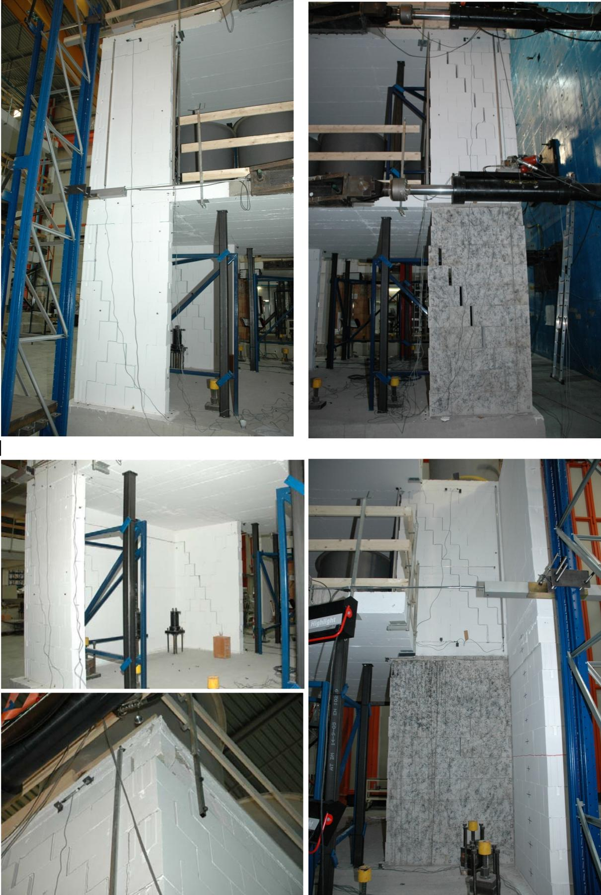
Figure 9: Damages in the calcium silicate specimen after the final test (0.20g)
