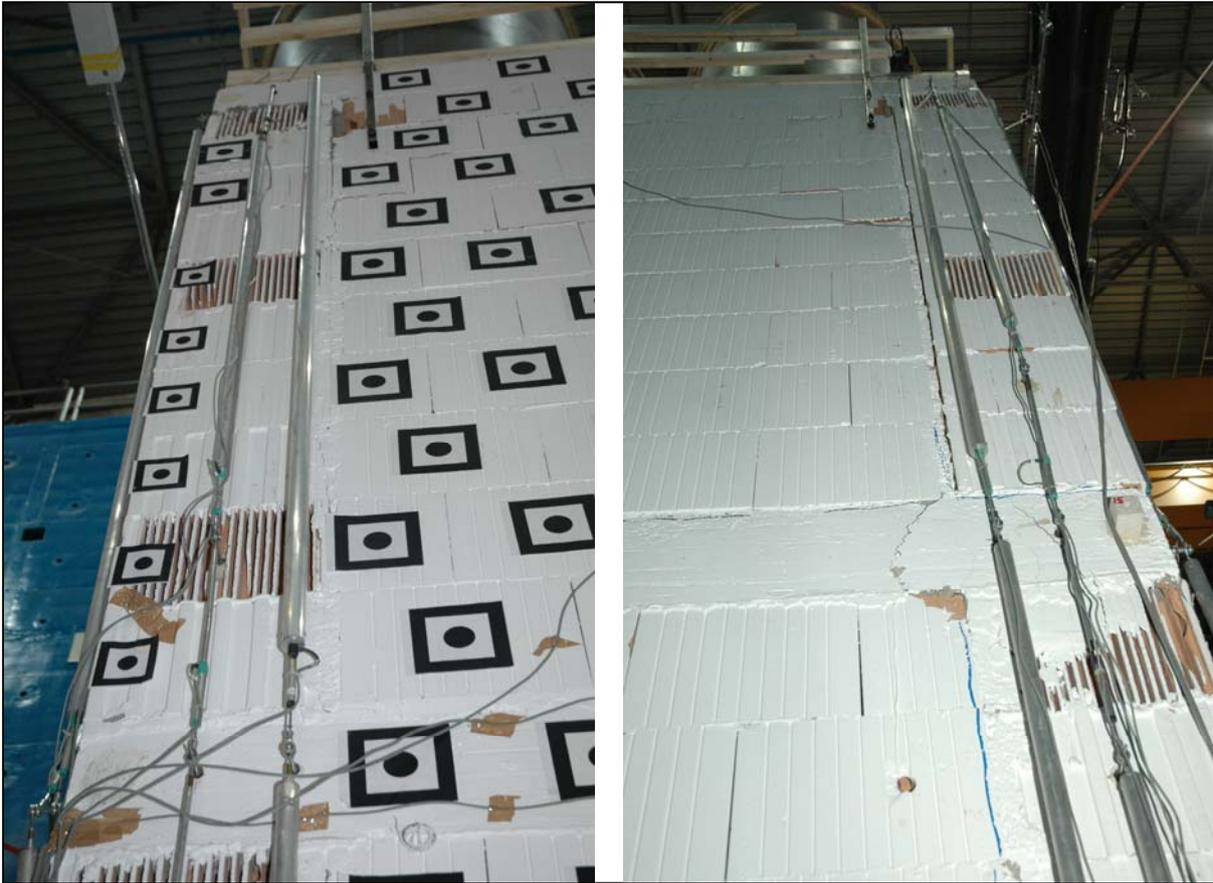
Figure 18: Damages in the slender walls junctions after the final test (0.22g)
