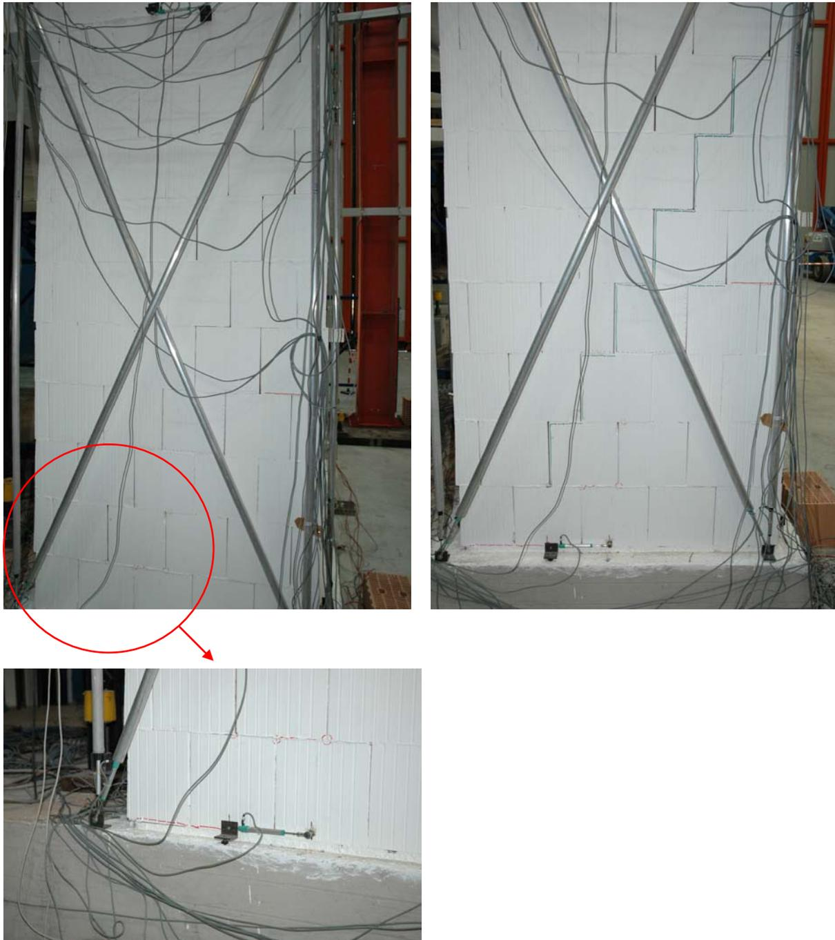
Figure 14: Cracks in the east slender wall of the ground floor after the 0.12g test (left) and the 0.14g test (right)
