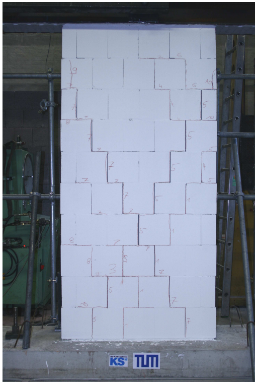
Figure 35: Crack pattern CS08
