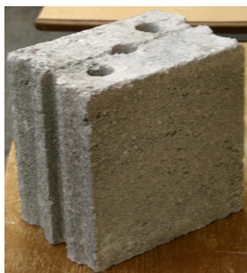
Figure 5: Lightweight Aerated Concrete units: Bisophon VBL- 12 - 2.0 6DF (175)
