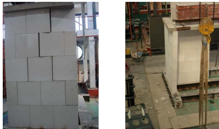
Figure 29. Specimen A3- with masses: Stepped cracks on transversal walls, permanent out of plane displacement.
