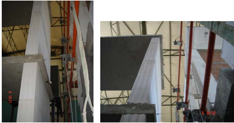
Figure 28. Specimen A3- without mass: Out of plane movements of transversal wall of 2 nd level.
