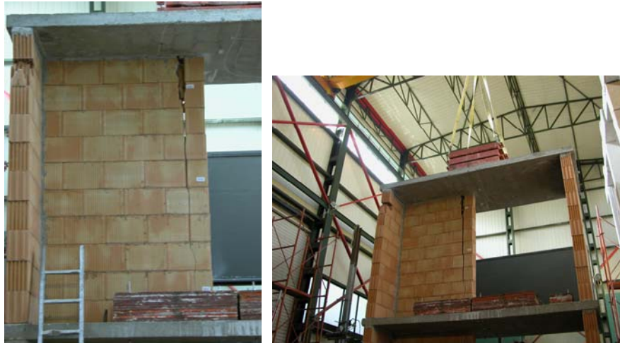
Figure 32. Specimen B2 - crack through the height of horizontal wall of 2 nd level.
