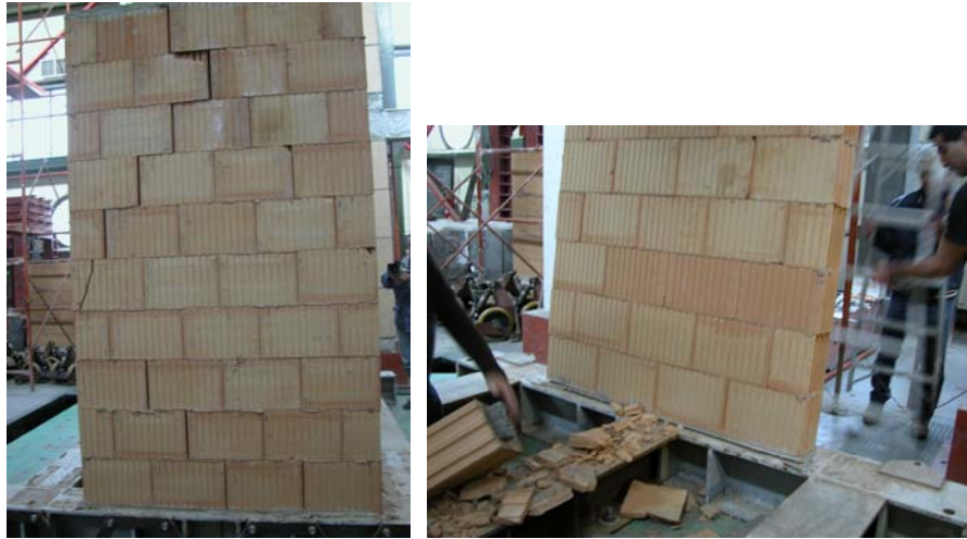
Figure 34. Specimen B2** : Cracks pattern of the transversal walls.
