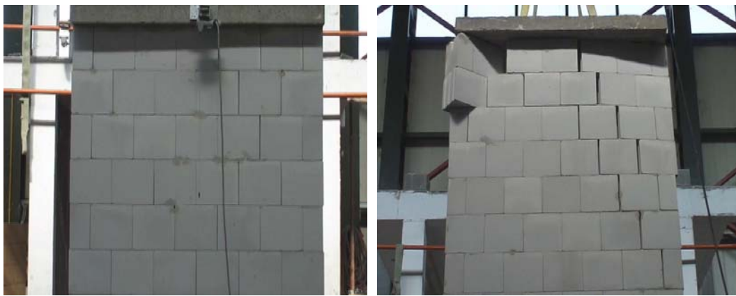
Figure 25. Specimen A1: Diagonal cracks of 1 st and 2 nd level in transversal wall, out of plane permanent displacement of wall at 2 nd level.
