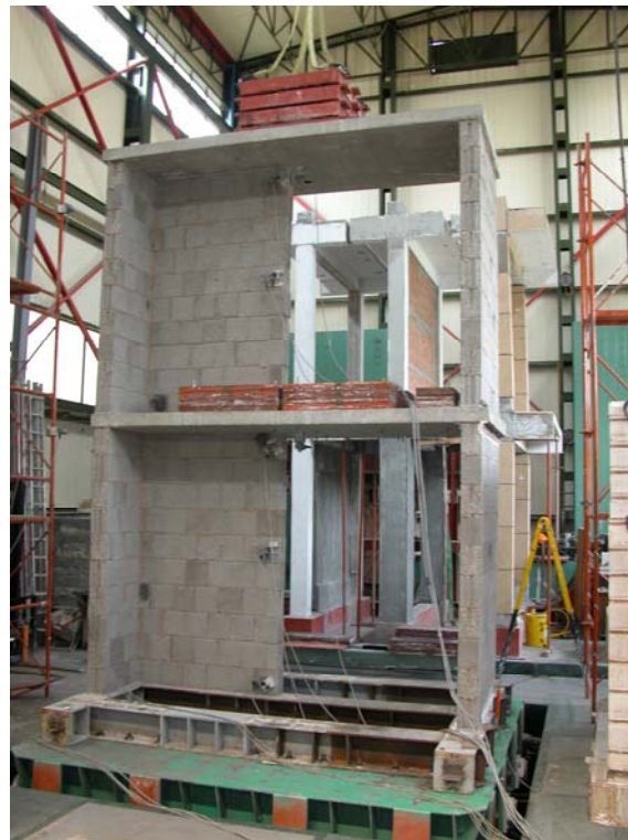
Figure 10. Specimen B4 with Lightweight concrete blocks.
