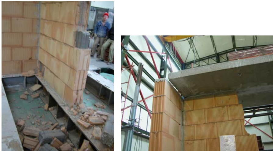
Figure 35. Specimen B2** : (a): Partial collapse of horizontal wall, (b): Permanent movement of plate.
