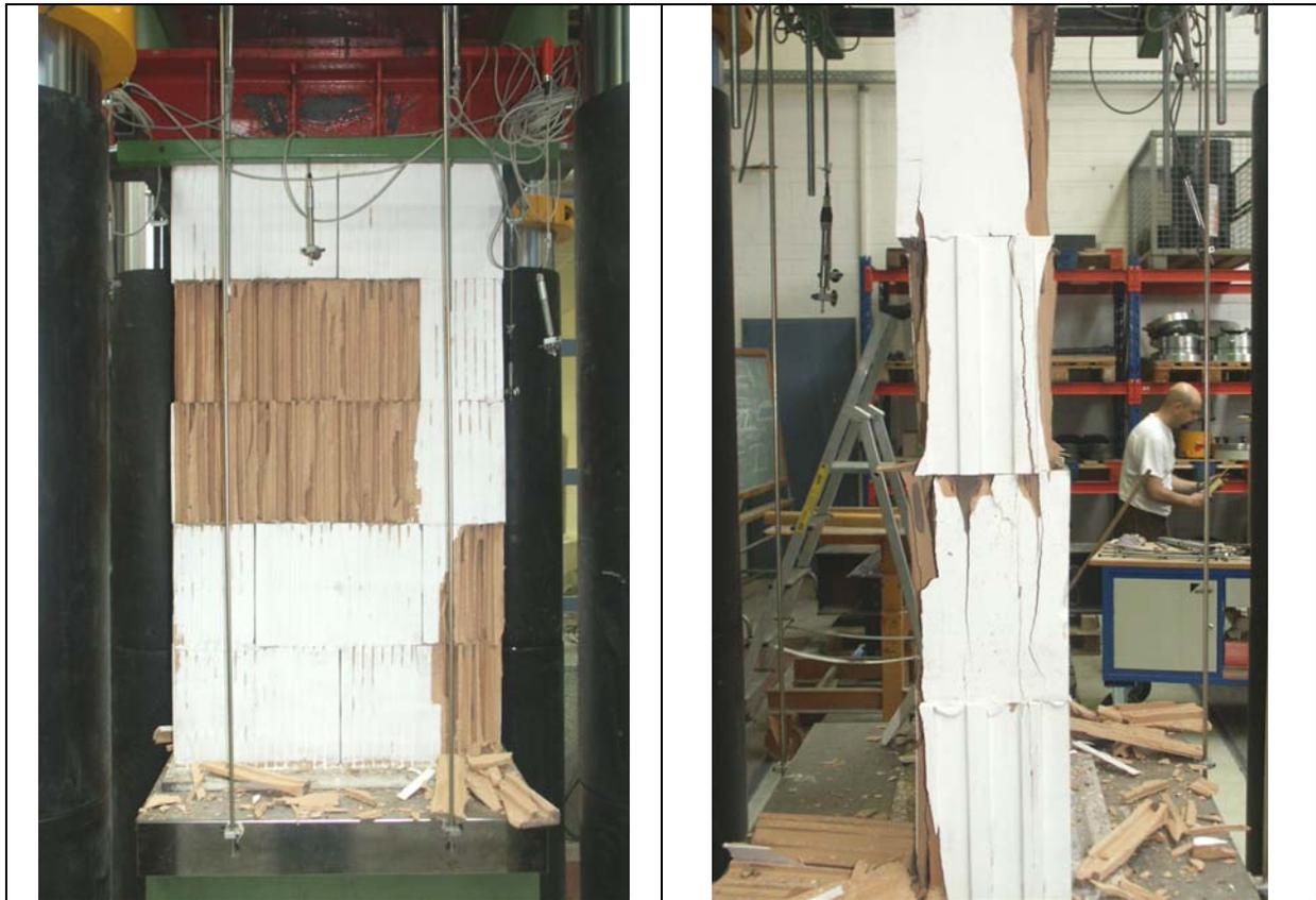
figure 4: destroyed specimen (Rilem\_2)
